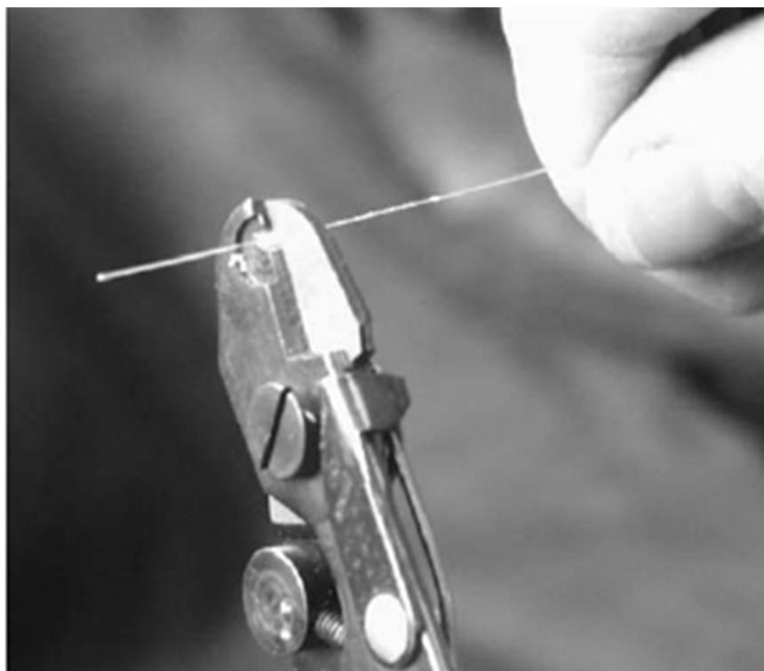
Figure 5-4. Using a stripping tool to remove the 250 micron Acrylate buffer from the fiber.
